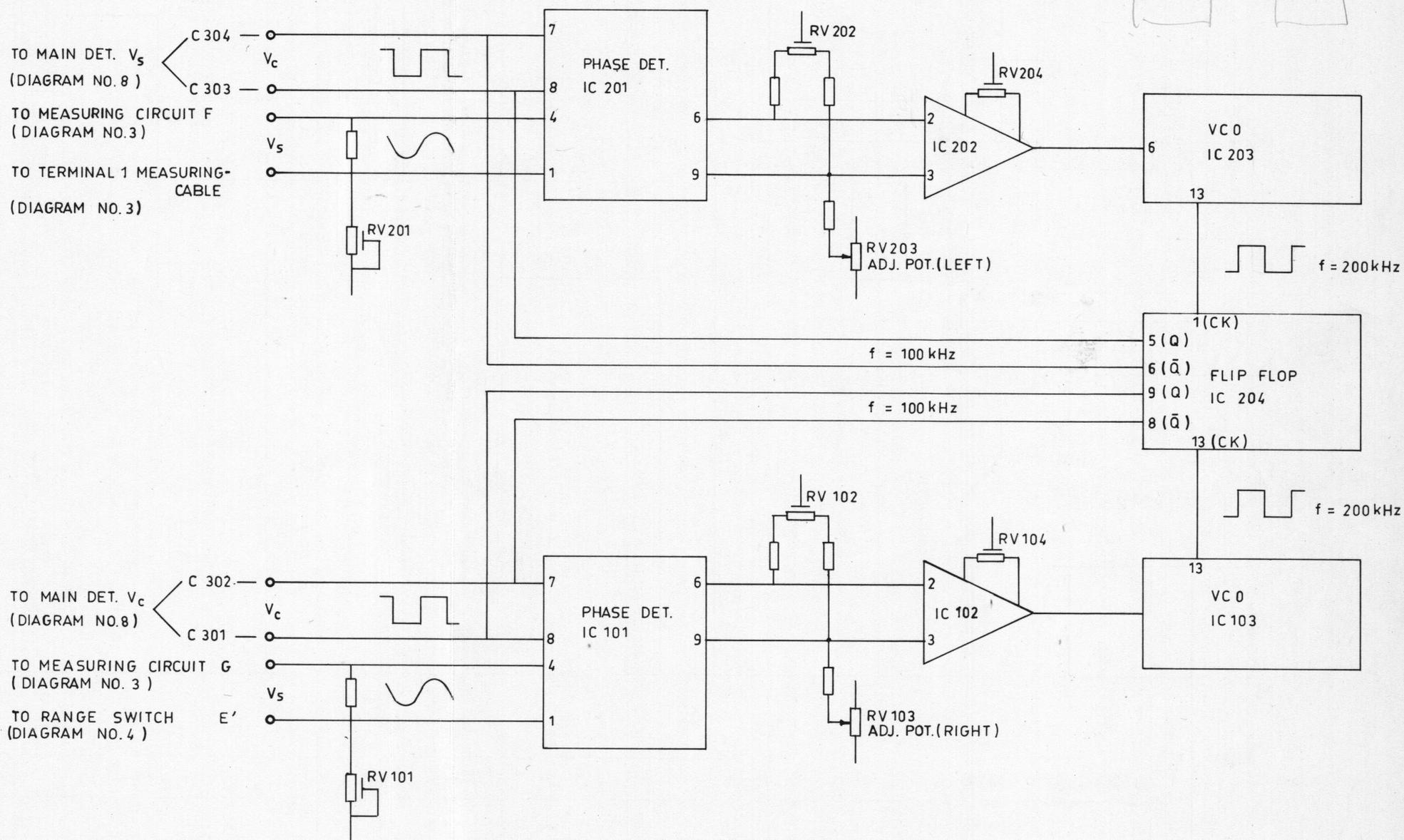
RV 103 and RV 203 is front panel multiturn potentiometers.
